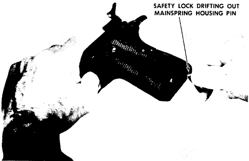
Figure 12. Hold the hammer, squeeze the trigger, and ease the hammer forward. Using the safety lock as a drift, press out the mainspring housing pin.
