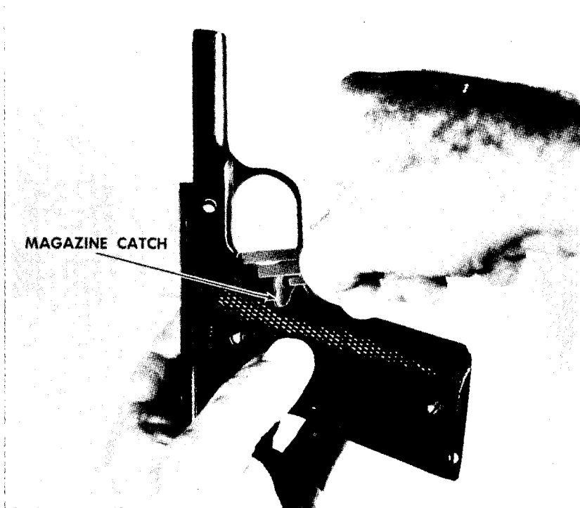
Figure 17. Press the magazine catch in until it is flush with the left side of the receiver. Using the short leaf of the sear spring as a screwdriver, turn the lock \frac{1}{4} turn counterclockwise. The lock should turn easily. If it does not check to see that the magazine catch is flush with the left side of the receiver. Force should not be used to turn the lock. Lift out the magazine catch. (Caution: Do not use the long leaf of the sear spring as a screwdriver.) To disassemble the magazine catch, turn the lock clockwise and separate the parts. Remove the trigger by elevating the front end of the receiver.
