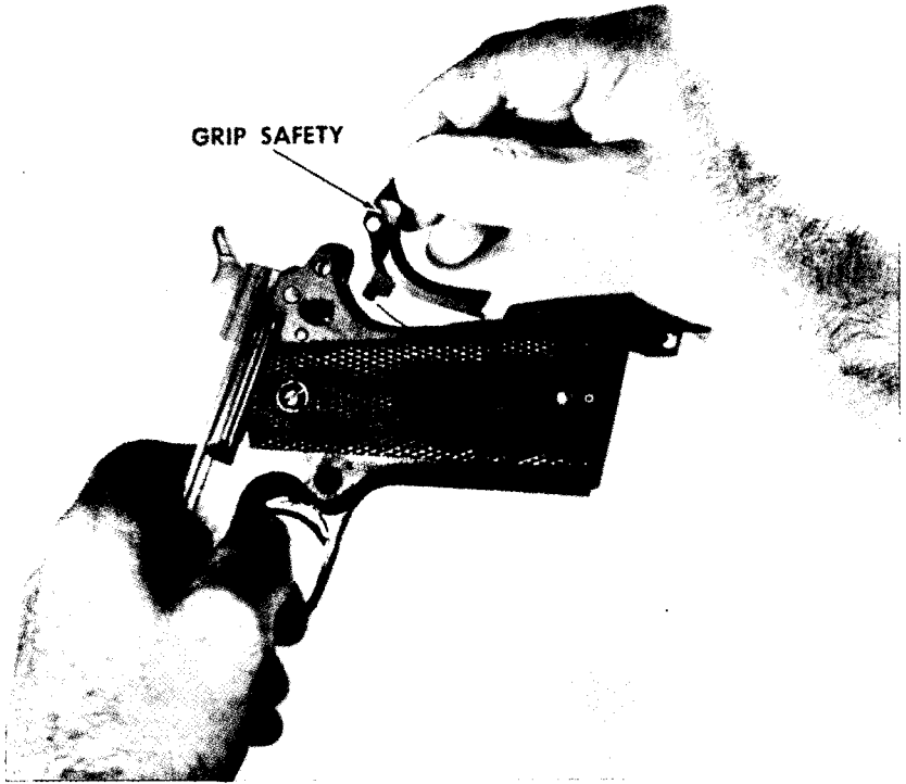
Figure 13. To remove the grip safety, slide the mainspring housing down about \frac{1}{2} inch and lift out the grip safety. Remove the mainspring housing by sliding it from the receiver. Disassemble the mainspring housing only when necessary for cleaning.
